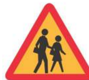
Figure 64. School zone ahead sign
